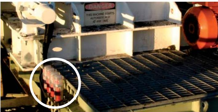
**Lubrication of various bearings on a coal crusher.** perma STAR made it possible to install the lubrication point outside the danger zone.
